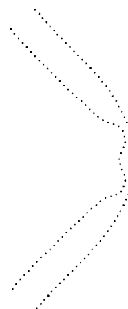
Fig. 2. The local buckling mode in the bending of a (10,10) carbon nanotube.
