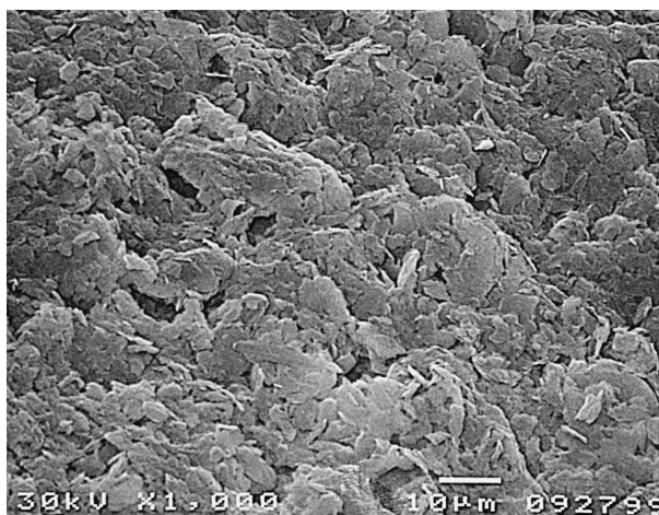
Fig. 5. SEM image (from above) of a spinning plate sample, with orientation factor 37.7, of talc, water/ethanol and epoxysilane. The individual tablets form a larger-scale overall orientation.
